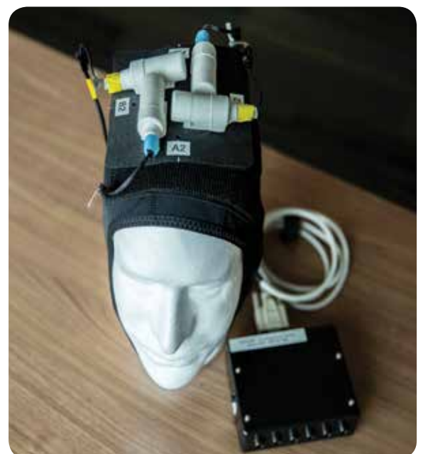
Portable TMS device that delivers stimuli at multiple cortical sites.
